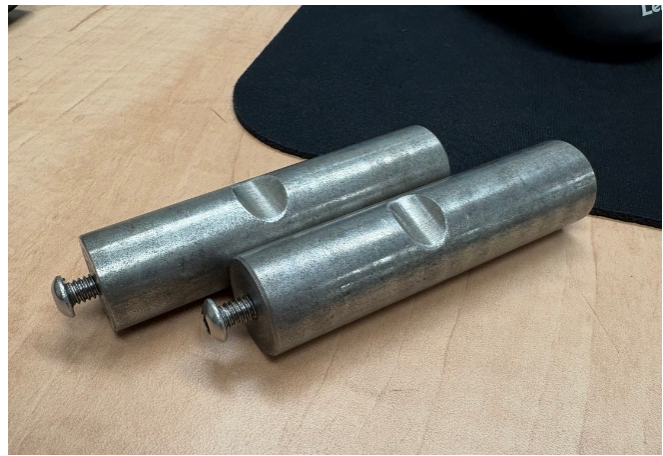
Fig. 1. Custom saddle-shaped support pins
